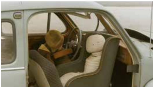
1964 - prototype car seat with test dummies
